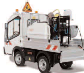
▼ Electric watering and spraying system
