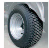
Tyres : Low pressure turf tyres 23x8,5x12
